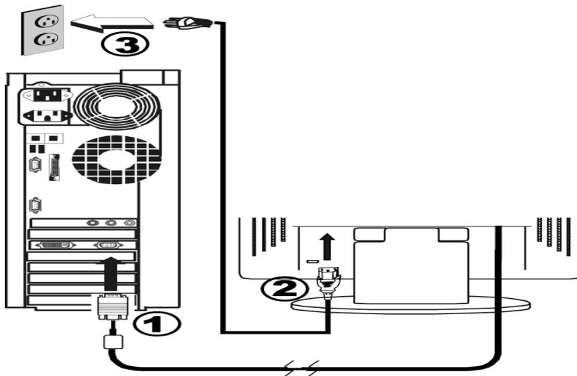
1. Connect the built-in video cable into the 15-pin connector on the back of your computer and tighten the two screws.
