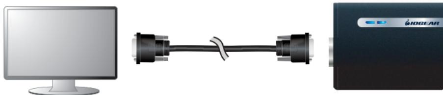
3. Connect the power adapter to the DVI Net ShareStation and make sure it is powered on. When the Link indicator lights up, the DVI Net ShareStation is correctly connected to the network.
