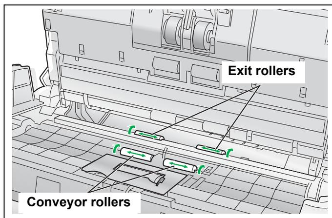
**8** Use the Roller Cleaning Paper to clean the surface of the free rollers.
