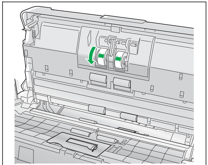
**7** Use the Roller Cleaning Paper to clean the surface of the conveyor rollers and exit rollers.
