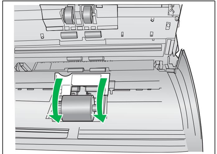
**6** Use the Roller Cleaning Paper to clean the surface of the double-feed prevention roller.
