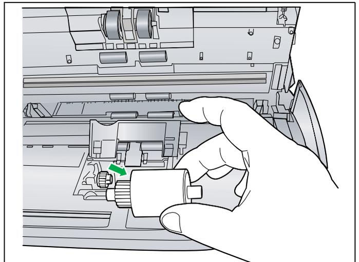
**5** Open the optional Roller Exchange Kit (KV-SS030), and retrieve a new paper feed roller.
