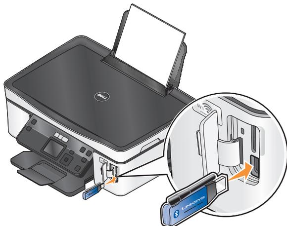
Bluetooth Dongle Connected appears on the display.
