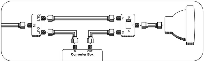
When the A/B switch is in the A position, you need to change channels on the converter box (and your TV should be tuned to channel 3 or 4); when the A/B switch is in the B position you can change channels on the TV.
