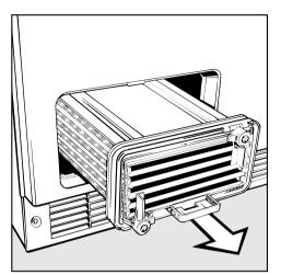
Pull out the heat exchanger
