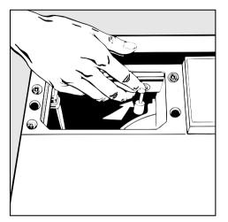
Close the water inlet port above the condensed water container with the bottom part of the rubber plug. The plug must face towards the interior of the machine so that the condensed water container can easily be inserted. Connection to wash basin drain outlet
