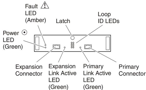
**Figure 1-6 LCC Connectors and LEDs**
