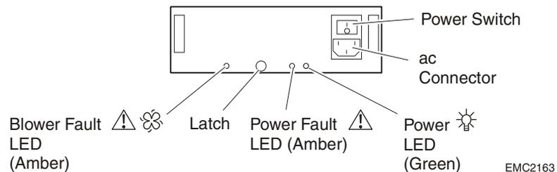
**Figure 1-8 Power Supply/System Cooling Module**
