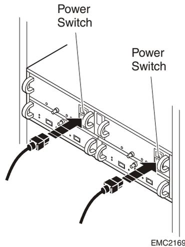
**Figure 2-2 Plugging in the ac Line Cord**
