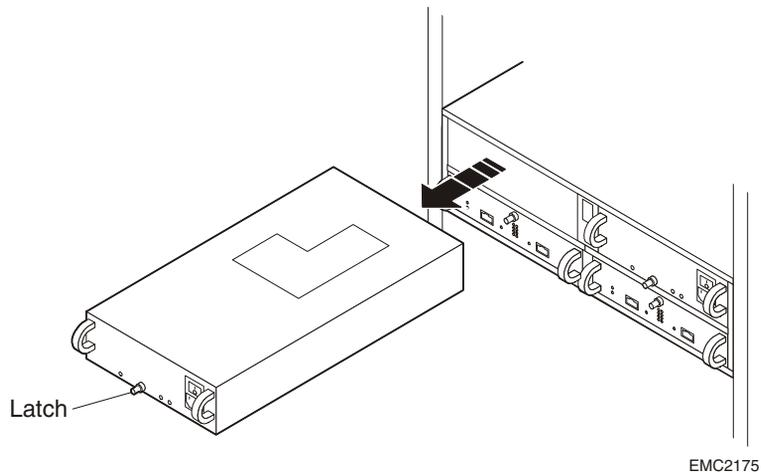
**Figure 3-16 Removing a Power Supply/System Cooling Module**
