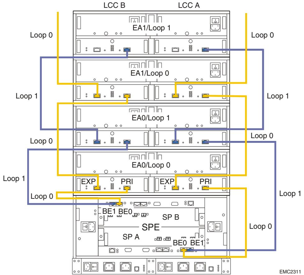
Figure 3-14 Connecting Disk Enclosures Together with Copper Cable
