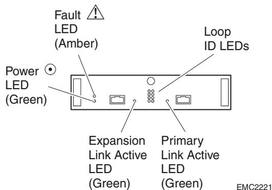
**Figure 3-4 LCC Status LEDs**
