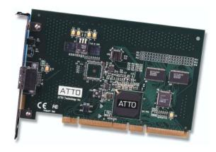
1.0625-Gigabit Fibre Channel Host Adapter With a Fixed Copper HSSDC Interface
