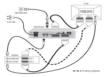
Screw the adapter supplied with your receiver on the "RF IN" connector of the rear panel. Use the antenna cord type F-IEC supplied to connect your receiver to the VCR/DVD. Use the SCART cable supplied to connect your receiver to the TV set.
