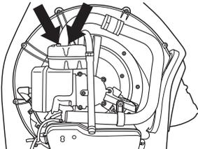
Pull out the spark arrestor mesh and clean using a wire brush. Replace the spark arrestor mesh if it is defective.
