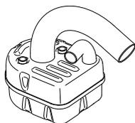
In countries that have a warm and dry climate there is a significant risk of fire. Consequently, we have equipped the muffler with a spark arrester mesh mounted inside the muffler.
