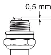
**CAUTION!** Always use the recommended spark plug type! Use of the wrong spark plug can damage the piston/cylinder.
