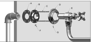
The adjustable flange allows for correct installation without the need for precise positioning of the internal pipe work. Therefore, the NPT connector should protrude from the wall / tile face 0 - 1/2".
