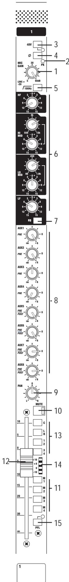
MIC GAIN (1) adjusts the sensitivity of both mic (XLR) and Line (1/4" jack) inputs. Both inputs are electronically balanced, and are located on the rear connector panel.
