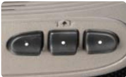
This programmable transmitter can store three frequencies for items such as a garage door opener, entry door lock or security system.
