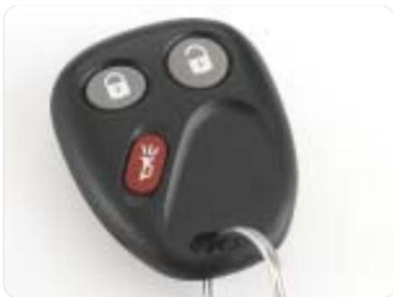
On equipped vehicles, the RKE system locks and unlocks the doors and liftglass from a range of three to 30 feet. At times the range may be shorter than usual, which is normal. If the transmitter does not seem to be working properly:
