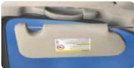
To block the sun's glare, pull the sun visor down. You can cover the driver or passenger front-side window by sliding the sun visor front-to-rear of vehicle and vice versa.
