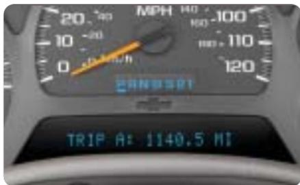
The DIC display is located above the steering wheel on the instrument cluster, and can be programmed in three languages. The controls are located on the steering wheel:
