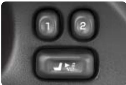
The memory seat controls are located on the driver door. They program and recall driver seat position and outside mirror settings for up to two drivers.
