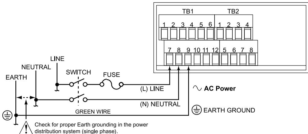
**Figure 3-8 Main Power Connections (ac powered unit)**
