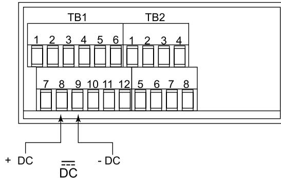
**Figure 3-9 Main Power Connections (dc powered unit)**
