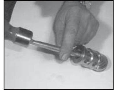
3. Valve seats (51C and 52C) are pressed out of spacer pipe (51F) by hitting the valve plate (51D) with a bolt.
