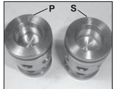
5. When reassembling: The suction valve seat (51C) is 1mm smaller in diameter than the discharge valve seat (52C). Suction valve seats are marked "S" and always have to be installed first. Discharge valve seats are marked "P" and are always to be installed on top of suction valve. Plugs (58) are to be tensioned down evenly with screws (58C) and crosswise at 156 ft-lbs. (210 NM).
