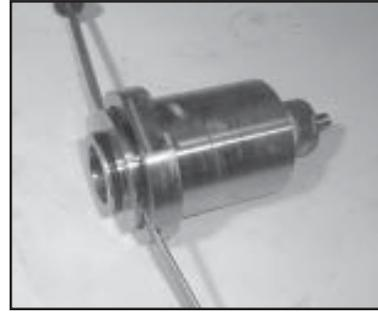
9. Pull seal sleeves (39) out of their fittings in the crankcase. Take seal case (38) out of seal sleeve (39).
