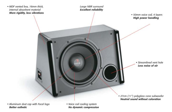
27cm (11") subwoofer Height: 310mm (12-3/16") Depth: 371mm (14-5/8") Length: 466mm (18-1/3") Max. Power: 500W
