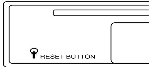
The RESET button is located on the front of main panel. It is recessed in order to prevent accidental engagement, and can be activated with the tip of a ball-point pen or any similar pointed object. This reset circuitry is provided in order to protect the unit's microprocessor, and should only be activated under the following conditions :
