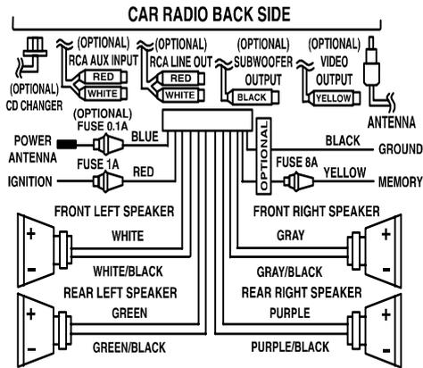
**CAUTION :** Do not connect the speaker wires to chassis or car body. Each speaker wire cannot be soldered together with other wires. Otherwise, the unit will be damaged and no sound will come out anymore.
