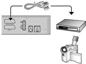
You can connect additional devices such as decoders, satellite receivers, camcorders, etc. to the *EURO AV2* socket. When playback is started on this additional device the DVD recorder automatically connects the *EURO AV2* scart socket with the *EURO AV1* scart socket. You will then see the picture from the additional device on your TV set, even if the DVD recorder is switched off.
