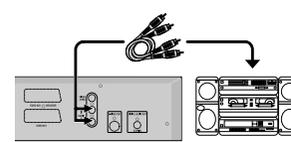
Two analogue audio sockets *AUDIO L/R* (audio signal output left/right) are located at the back of the DVD recorder.
