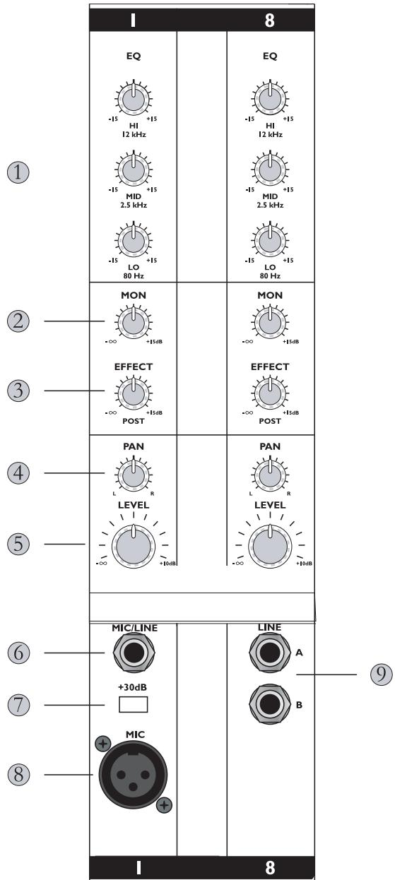
1. **Equalizer controls** enable you to shape the sound of the channel before it is sent to the outputs.
