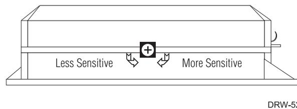
There is a dual-stage shock sensor inside the control unit. Adjustments are made via the rotary control as indicated in the diagram. Since the shock sensor does not work well when mounted firmly to metal, we do not recommend screwing down the control module. The full trigger of the on-board shock sensor reports *Zone 2*. (See *Table of Zones* section of this guide.)
