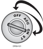
2. **Ignition.** Turn the ignition on, then back off: (The H1/9 YELLOW wire must be connected.)
