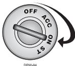
2. **Turn the ignition on.** (The YELLOW wire, H1/9 must be connected.)
