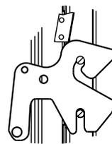
4. Insert the door stop clip with the angular surface at the top of the frame hinge slot, then push in the bottom of the clip until flanges are flush with the front frame.
