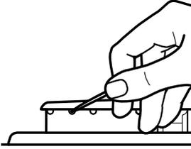
4. Replace the burner cap, making sure the alignment pins on the cap are properly aligned with the burner base.
