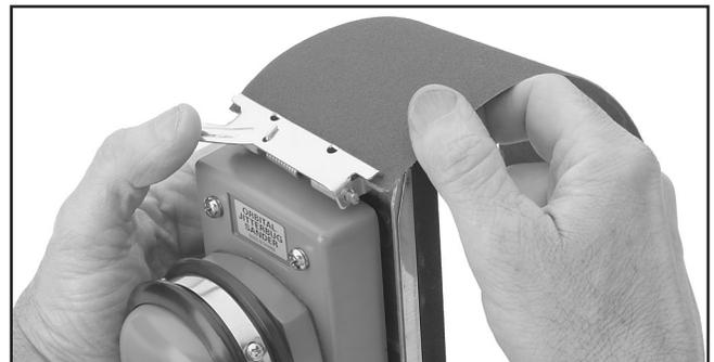
Figure 2. Attaching sanding sheet.
