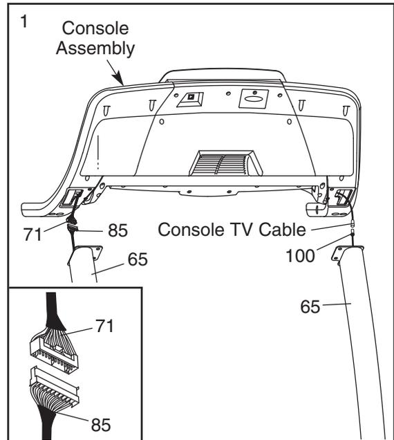
2. Insert the slack in the Wire Harnesses (71, 85) and the console TV cable into the Uprights (65).
