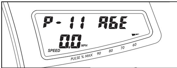
If heart rate program 11 is selected, a pulse symbol will scroll across the matrix in the left display. If heart rate program 12, 13, or 14 is selected, a profile of the target heart rate settings of the program will appear in the matrix in the left display.
