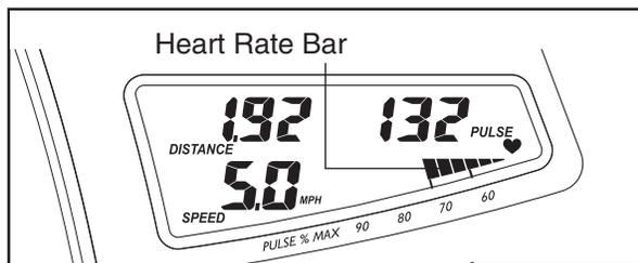
Note: The console can display speed and distance in either miles or kilometers. The letters "MPH" or "Km/H" will appear in the right display to show which unit of measurement is selected. To change the unit of measurement, see *HOW TO USE THE INFORMATION MODE* on page 20. **For simplicity, all instructions in this section refer to miles.**
