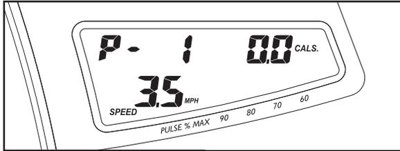
When a preset program is selected, the left display will flash the maximum incline setting of the program for a few seconds, and the right display will flash the maximum speed setting. The left display will then show how long the program will last. In addition, the first ten speed settings of the program will appear the matrix in the left display.
