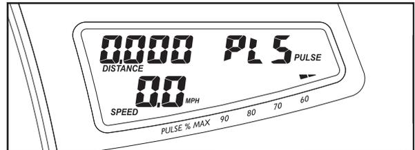
If heart rate program 12, 13, or 14 is selected, the letters “PLS” and the maximum target heart rate setting for the program will begin to flash in the right display. If desired, change the maximum target heart rate setting by pressing the + or – button beside the Enter button (see EXERCISE INTENSITY on page 25). Then, press the Enter button. Note: If the maximum target heart rate setting is changed, the intensity level of the entire program will change.
