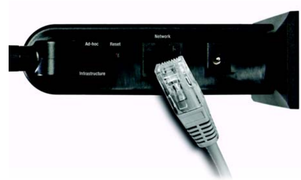
Figure 5-1: Connect the Ethernet Network Cable
