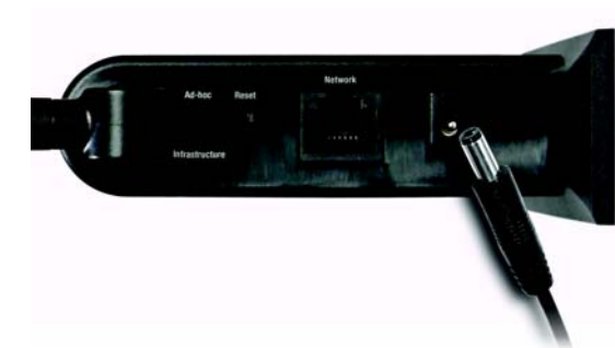
Figure 4-2: Connect the Power
