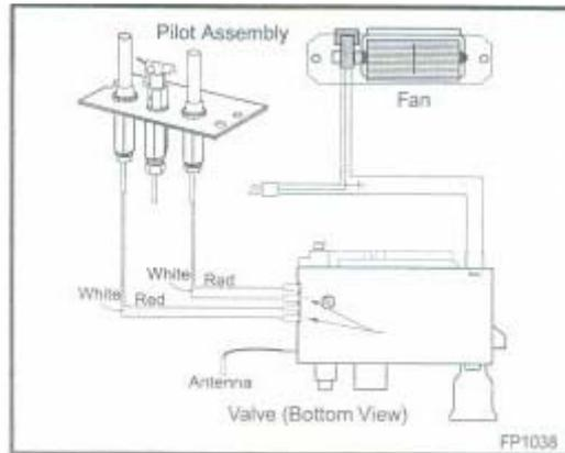
Fig 8. Comfort control wiring diagram
