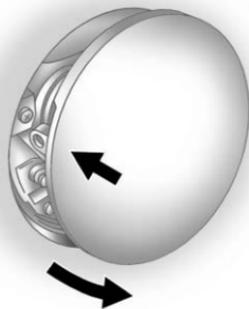
The tethered fuel cap is located behind a hinged fuel door on the passenger side of the vehicle.
