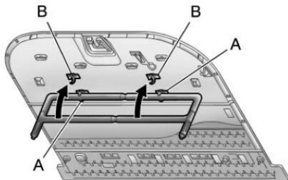
3. Insert the top of the fence into the lower two clips (A).
