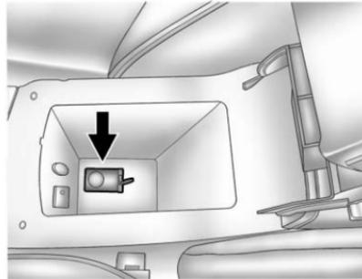
2. Place the transmitter in the transmitter pocket.
