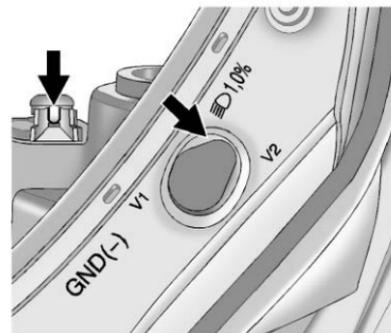
7. Locate the vertical headlamp adjusters, which are under the hood near each headlamp assembly.
