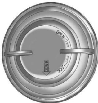
1. From the back side of the headlamp assembly, remove the bottom cap to replace the DRL bulb.
