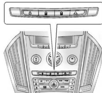
The power door lock switches are on the instrument panel.
