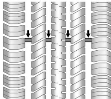
One way to tell when it is time for new tires is to check the treadwear indicators, which appear when the tires have only 1.6 mm (1/16 in) or less of tread remaining.
