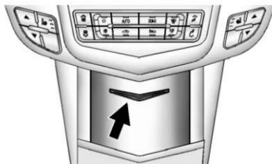
A storage area is located in front of the shift lever. Push upward on the top of the door and release; the door automatically opens.
