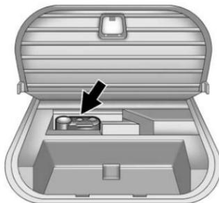
This vehicle may have a tire sealant and compressor kit in place of a jack or spare tire. It is located in a foam container in the rear compartment storage area. If the vehicle has a cargo cover, see *Cargo Management System* on page 4-5 for instructions on how to access the tire sealant and compressor kit.
