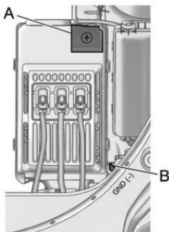
Your vehicle is equipped with a remote positive (+) terminal (A) and a remote negative (-) terminal (B). The remote
