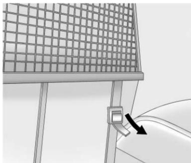
6. Pull on the straps to tighten the net.
