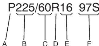
**(A) Passenger (P-Metric) Tire:** The United States version of a metric tire sizing system. The letter P as the first character in the tire size means a passenger
