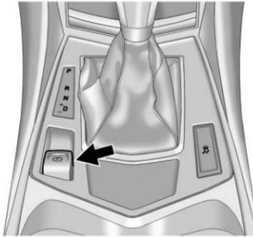
The vehicle has an Electric Parking Brake (EPB). The switch for the EPB is in the center console. The EPB can always be activated, even if the ignition is OFF. To avoid
