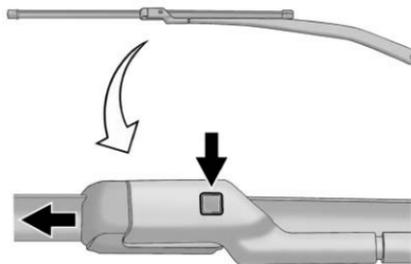
2. Press the button in the middle of the wiper arm connector, and pull the wiper blade away from the arm connector.
