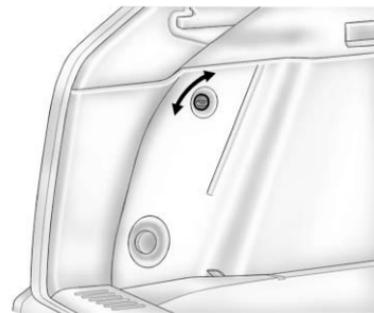
The rear compartment fuse block is located in the cargo area, on the driver side of the vehicle behind the lower trim panel. To open, turn the latch with a flat bladed tool and pull the trim panel from the edges to fold it down.
