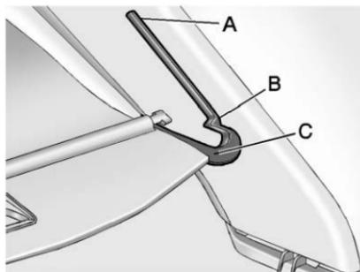
5. Insert the shade's pins in the channels (C) on both sides.
