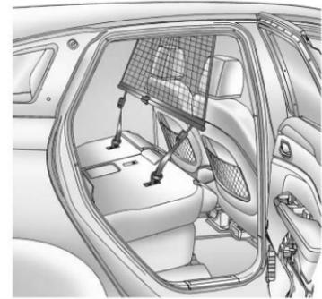
3. Mount the cargo net to the rear seat tethers located on the back of the folded down rear seats and pull on the straps to tighten the net.
