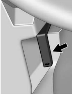
1. Pull the release handle with the above symbol on it. It is located below the instrument panel to the left of the steering wheel.
