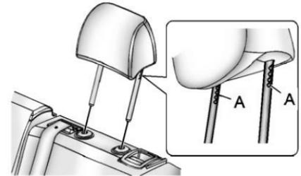
1. Insert the head restraint posts into the holes in the top of the seatback. The notches (A) on the posts must face the driver side of the vehicle.
