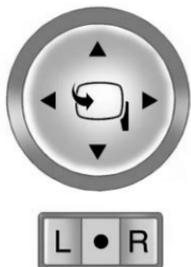
Vehicles with power folding mirrors have controls on the driver door.
