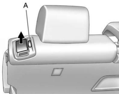
3. Lift the lever on the top of the seatback. The rear seatback lock indicator (A) extends when the seatback is unlocked.
