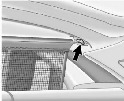
1. Insert the top corners of the cargo net into the large opening in the headliner and secure by sliding them into the small opening.
