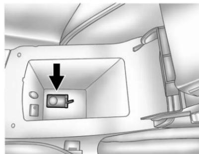
4. Place the new transmitter into the transmitter pocket. The transmitter pocket is inside the center console storage area located between the driver and front passenger seats. The storage area will need to be opened and the storage tray lifted up to access the transmitter pocket.
