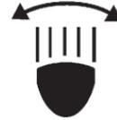
This light comes on solid when there is a problem with the Adaptive Forward Lighting system and flashes when the system is switching between lighting modes. See *Adaptive Forward Lighting (AFL)* on page 6-3 for more information.
