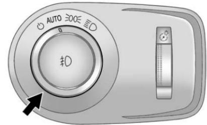
The exterior lamps control is located on the instrument panel to the left of the steering column.
