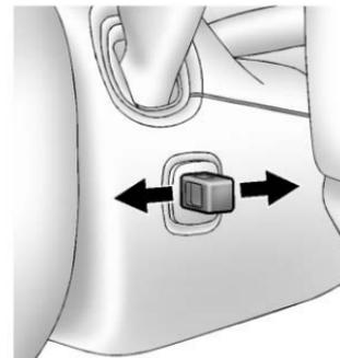
The switch used to adjust the pedals is located on the right side of the steering column, below the wiper stalk. Pull the switch toward you to move the pedals further from the floor, or push the switch away from you to move the pedals closer to the floor.
