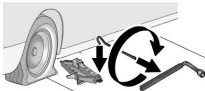
7. Insert the hooked end of the extension handle through the jack and the flat end through the wheel wrench.
