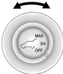
On vehicles with a power liftgate the switch is located on the driver door. The vehicle must be in P (Park) to use the power feature. The taillamps flash when the power liftgate moves.
