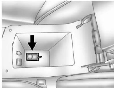
3. Place the new transmitter into the transmitter pocket. The transmitter pocket is inside the center console storage area located between the driver and front passenger seats. The storage area will need to be opened and the storage tray lifted up to access the transmitter pocket.
