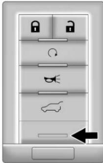
To remove the key, press the button near the bottom of the transmitter, and pull the key out. Never pull the key out without pressing the button.
