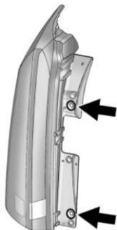
4. Remove the two screws from the taillamp assembly.
