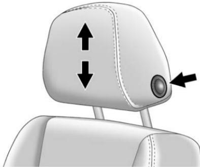
1. To raise or lower the head restraint, press the release button while pulling up or pushing down on the head restraint.
