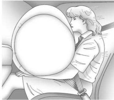
The right front passenger frontal airbag is in the instrument panel on the passenger side.
