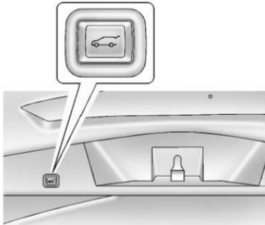
Press and release
