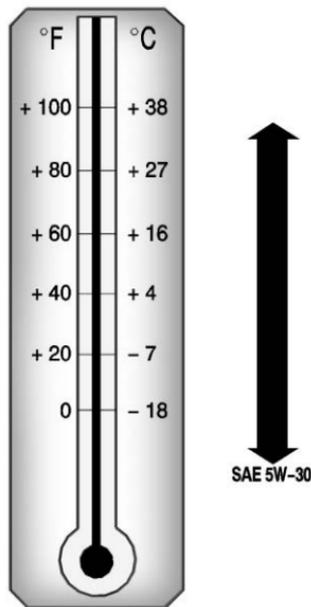
Cold Temperature Operation: In an area of extreme cold, where the temperature falls below  $-29^{\circ}\text{C}$  ( $-20^{\circ}\text{F}$ ), an SAE 0W-30 oil should be used. An oil of this viscosity grade will provide easier cold starting for the engine at extremely low temperatures. When selecting an oil of the appropriate viscosity grade, be sure to always select an oil that meets the required specification, dexos™. See "Specification" for more information.
