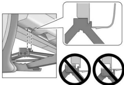
9. Raise the vehicle by turning the wheel wrench clockwise until the slots in the jack head fit into the metal flange located behind the triangle on the plastic moulding.
