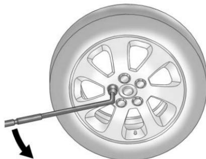
4. Turn the wheel wrench counterclockwise to loosen all the wheel nuts, but do not remove them yet.
