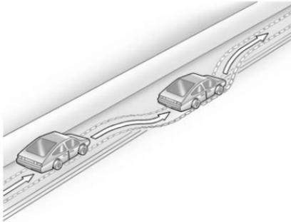
If the level of the shoulder is only slightly below the pavement, recovery should be fairly easy. Ease off the accelerator and then, if there is nothing in the way, steer so that
