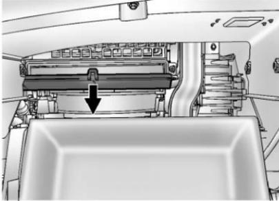
4. Release the two latches holding the service door. Lower the service door.
