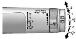
The windshield wiper/washer lever is located on the right side of the steering column. With the ignition in ACC/ACCESSORY or ON/RUN/START, move the windshield wiper lever to select the wiper speed.
