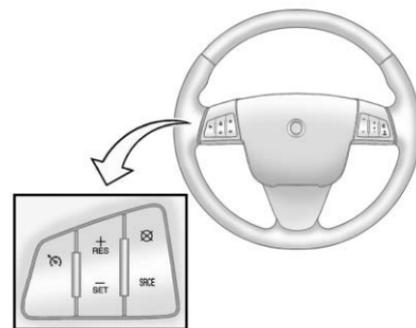
**Cruise Control** : Press to turn cruise control on and off.
