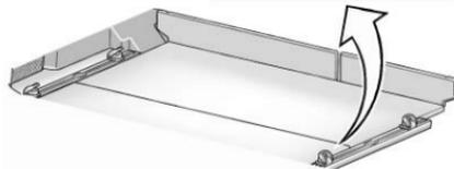
The loop of the D-ring slider must be facing inward towards the storage area and the ring must be in the up position for proper usage.
