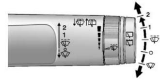
The windshield wiper/washer lever is located on the right side of the steering column. With the ignition in ACC/ACCESSORY or ON/RUN/START, move the windshield wiper lever to select the wiper speed.
