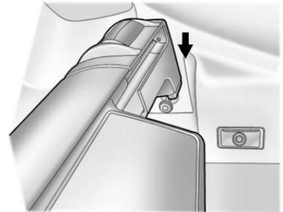
2. Align the cartridge over the pins on the trim panels of the vehicle.
