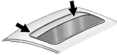
Dirt and debris may collect on the sunroof seal or in the track. This could cause an issue with sunroof operation, noise, or plugging the water drainage system. Periodically open the sunroof and remove any obstacles or loose debris. Wipe the sunroof seal and roof sealing area using a clean cloth, mild soap, and water. Do not remove grease from the sunroof.
