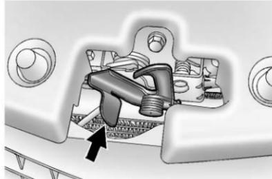
2. Move the secondary hood release lever up to release the striker. The lever is located near the middle of the hood.
