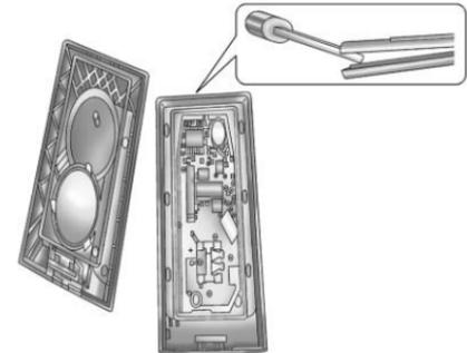
2. Use the key blade to separate the two halves of the transmitter.
