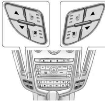
If available, the buttons are near the climate controls on the instrument panel. To operate, the ignition must be in ON/RUN/START.
