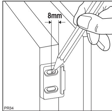
Remove the little plates and make the holes with a diam. of 2 mm. Replace the little plate over the runners and screw in the screws provided (3.5x16 mm). For the alignment of the kitchen unit door, if necessary, use the clearance size of the slotted holes. At the end of the procedure, check that the doors of the appliance and the kitchen unit open properly.
