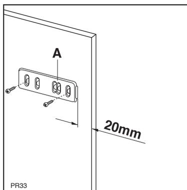
Open both the appliance door and that of the kitchen unit to approx. 90°. Place the little plates over the runners. Hold the doors of the appliance and the unit together and mark the holes.
