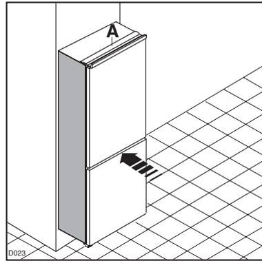
If after having carried out the previously described operation there is still some space left between the appliance and the kitchen unit, fit the trimming provided together with the appliance on the stop strip (A).
