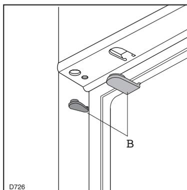
Position the runners (A) at the top and bottom of the inside of the kitchen unit as shown in Fig. and mark the position of the external holes.
