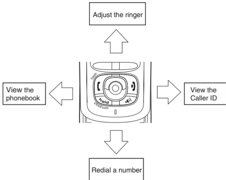
You will also use the joystick to make menu selections. To enter the menu, press in on the center of the joystick or press the Menu soft key.
