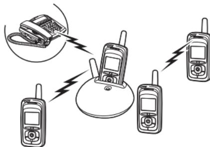
Press the **MENU** soft key, and select the Link Handsets option, then select DirectLink Mode. When the phone displays DirectLink by pressing center/select knob, press the center of the joystick. The phone displays In DirectLink Mode.
