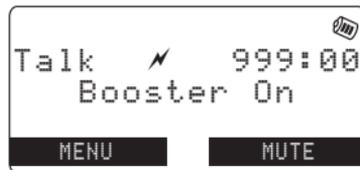
While you are on a call, press the center of the joystick and then select Clarity Boost. Boost On and ⚡ appear on the display. To turn off the Clarity Booster, repeat above steps again.
