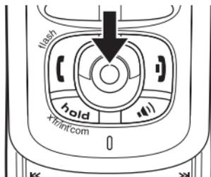
Select the highlighted option by pressing in on the center of the joystick. (You can also press the **OK** soft key.) Anytime the display prompts you to press **OK** or the **ENTER** soft key, you can press the center of the joystick.
