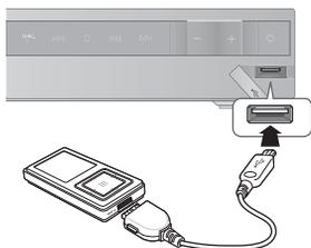
1. Connect the USB device to the USB port on the front panel of the product.
