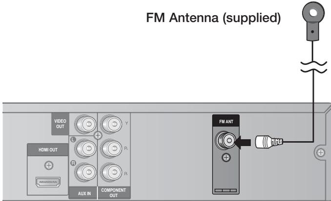
1. Connect the FM antenna supplied to the FM Antenna jack.
