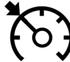
**Anti-theft system:** Flashes when the SecuriLock® Passive Anti-theft System has been activated.
