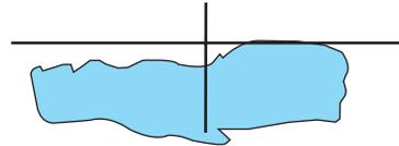
5. Locate the vertical adjuster on each headlamp. Using a Phillips #2 screwdriver, turn the adjuster either clockwise (to adjust down) or counterclockwise (to adjust up). The horizontal edge of the brighter light should touch the horizontal reference line. Close the hood and turn off the lamps.
