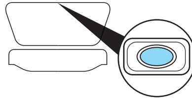
**Note:** For the best performance allow the power system to open the liftgate after pressing the control. Manually pushing or pulling the liftgate may activate the system's obstacle detection feature and stop the power operation.
