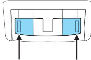
Your vehicle has second row lamps located within the grab handles. Press the lens up to turn on the lamps.
