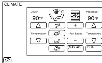
**Temperature**– Press the  $\Delta$  up and  $\nabla$  down arrows on the left side of the screen to increase/decrease the airflow temperature for the driver side of the vehicle. This control also adjusts the passenger side temperature when dual zone operation is disengaged.
