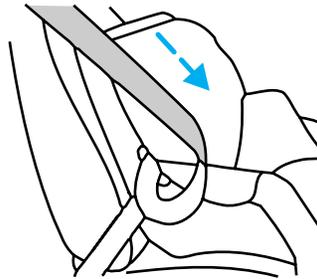
6. Allow the belt to retract to remove slack. The belt will click as it retracts to indicate it is in the automatic locking mode.
