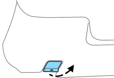
2. Go to the front of the vehicle and release the auxiliary latch using the handle that is located under the front passenger side of the hood.
