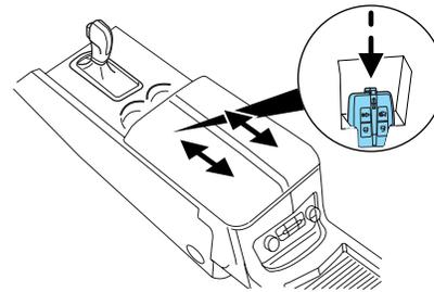
the backup slot, located in the rear of the center console utility compartment. Insert the IA key into the slot with buttons facing out and with key ring up. After inserting the IA key into the backup slot, use the START/STOP button and brake pedal to start your vehicle as usual. The vehicle should respond normally as long as the IA key is in the backup slot in the center console utility compartment. Once the vehicle is started, the IA key can be removed from the backup slot, if desired.
