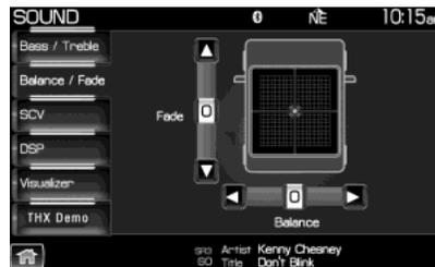
**SCV (Speed compensated volume):** With this feature on, the radio volume changes automatically with vehicle speed to compensate for road and wind noise. Select a level of compensation between 1 and 7 by pressing the corresponding button.
