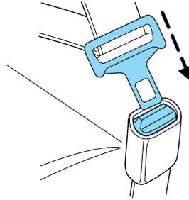
5. To put the retractor in the automatic locking mode, grasp the shoulder portion of the belt and pull downward until all of the belt is pulled out.
