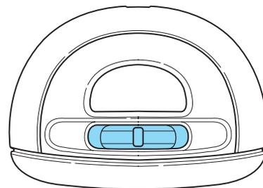
With the switch in the on position, the lamp will stay on all the time. In the off position, the lamp will stay off even when the doors are opened. With the switch in the center position, the lamp will turn on when the doors are opened and the top of the panel dimmer control is pressed to the full on position.
