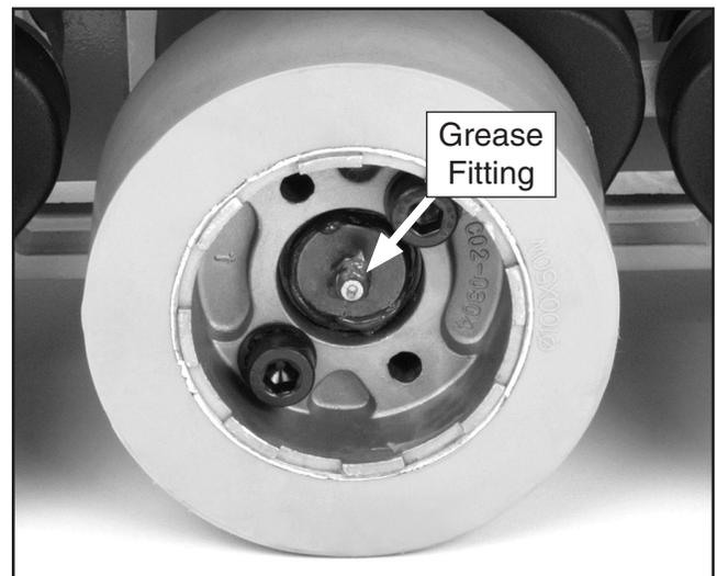
**Figure 13.** Wheel lubrication.
