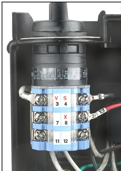
Figure 16. Motor power and direction switch.
