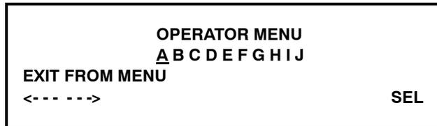
Screen "B" is FAULT DESCRIPTION. The fault description will indicate if there is a fault with the freezer and the side of the freezer where the fault occurred. To clear the tone for any faults which have been corrected, press the left arrow key. To see if there is more than one fault per cylinder, press the SEL key. When the last fault is displayed, the control will return to the OPERATOR MENU. To return to the main screen, move the cursor to "A" and press the SEL key again.
