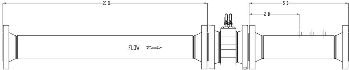
Figure 2-3 Piping recommendations bidirectional flow
