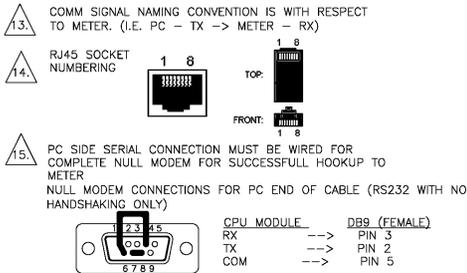
FEMALE 9 PIN DSUB CONNECTOR (BACK VIEW)
