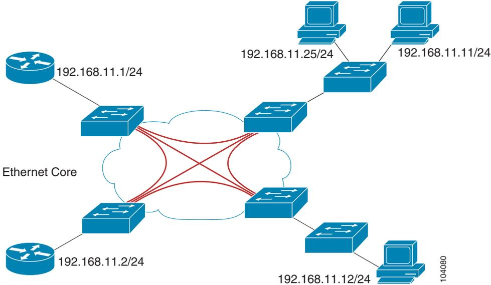
The Ethernet Relay Service (ERS or EVP-LAN) offers the any-to-any connectivity characteristics of EWS and the service multiplexing. This combination enables a single UNI to support a customer's intranet connection and one or more additional EVCs for connection to outside networks, ISPs, or content providers. Figure E-12 illustrates an ERS (EVP-LAN) VPLS multipoint topology.
