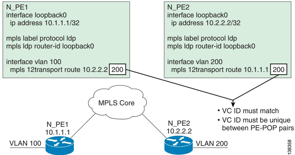
Note that the VC ID has to be the same on both ends of the EoMPLS tunnel. On each N-PE, there is mapping done between the VLANs to the EoMPLS tunnel. (See [Figure E-5](#).)
