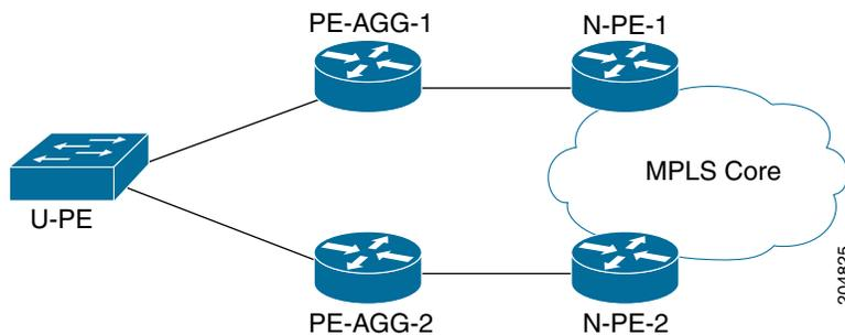
The first topology (N-PE redundancy starting at the U-PE, as shown in [Figure D-1](#)) provides the model of fault recovery for the N-PE device. As shown in the diagram, there are two different outgoing interfaces starting from the U-PE device. Each terminates at a different N-PE.
