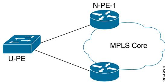
**Figure D-2 N-PE and PE-AGG Redundancy, Starting at the U-PE**
