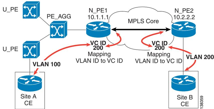
The VLAN IDs allocated and used at each access domain do not have to be the same.
