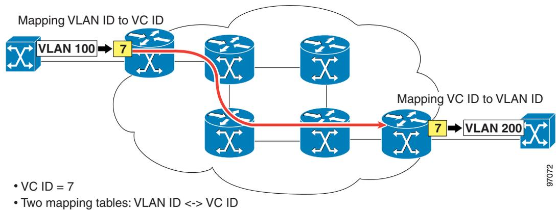
For the overall connection, this mapping is: VLAN ID <-> VC ID <-> VLAN ID.
