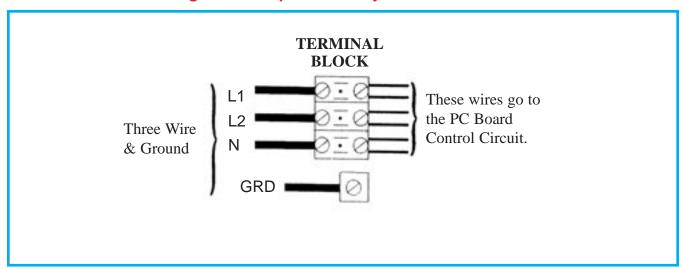
Connections should be made using copper conductors only. The connecting wire and circuit breakers or fuses must be sized to accommodate the total ampere load as specified on the equipment module data label.
