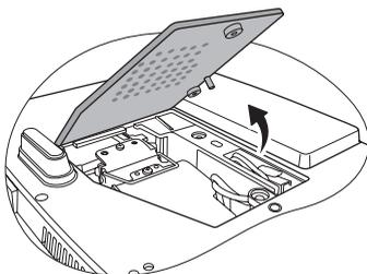
4. Loosen the screw that secures the lamp.
