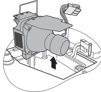
7. Insert the new lamp into the lamp compartment and make sure it fits in the projector.
