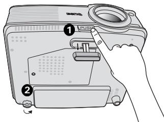
If the projector is not placed on a flat surface or the screen and the projector are not perpendicular to each other, the projected image becomes trapezoidal. To correct this situation, see "[Correcting keystone](#)" on page 30 for details.
