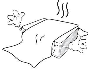
If the ventilation holes are seriously obstructed, overheating inside the projector may result in a fire.
