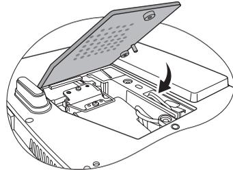
12. Tighten the screws that secure the lamp cover.
