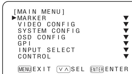
This display appears when the MENU/EXIT button is pressed. If no further action is taken for the next 120 seconds, the display will be automatically cleared.
