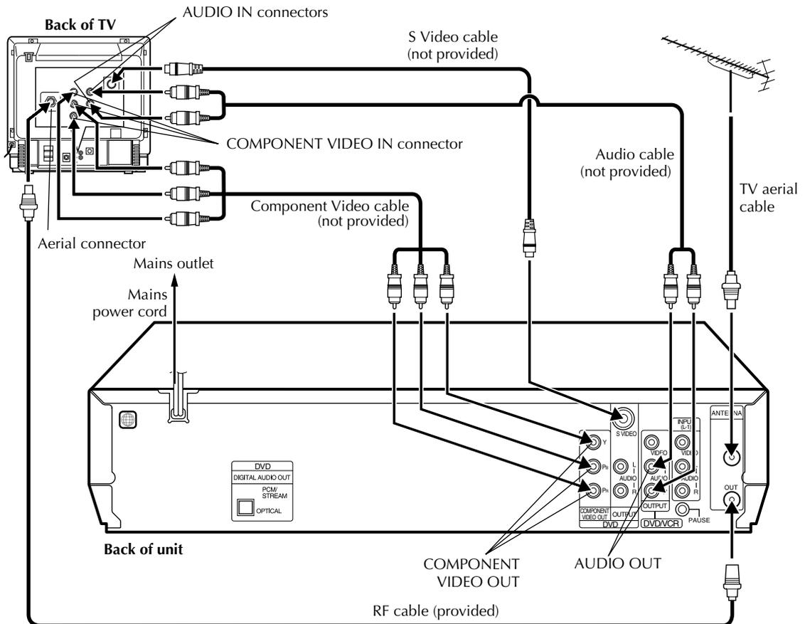
■ To connect to a TV with COMPONENT VIDEO IN connectors . . .
