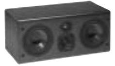
M6 - Designed for medium to large rooms. The high output M6 is a 3-way, acoustic suspension, magnetically shielded monitor employing (2) 6.5" woofers, a 4" midrange and a 1" aluminum dome tweeter.
