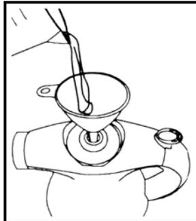
**WARNING:** This appliance is under pressure. After every use, press trigger button until all pressure has been released before removing safety cap.
