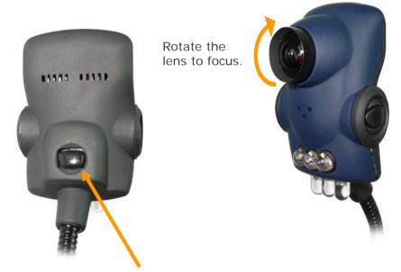
Press this button to switch the white LEDs on; press again to switch off.
