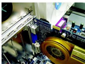
4-3-3 Insert the interface card into the expansion slot with care.
