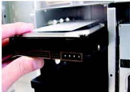
4-8-1 Use the runners installed on both sides of the HDD evenly and slide the HDD into the hard disk drive bay.
