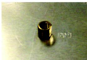
4-2-1 According to motherboard specifications, select proper screw holes, engage the standoffs into the corresponding holes of the casing.
