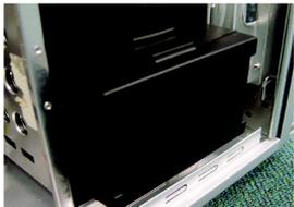
4-8-2 For installation of the fourth and fifth HDDs, loosen the tool enclosure, and then install the HDD in accordance with Step 4-8-1.
