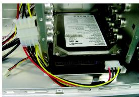
4-8-3 In case the length of power cable is not sufficient for installation of the bottom HDD, it is possible to use the power extension cable inside the tool enclosure, depending on the HDD with 4-pin or SATA power cable.
