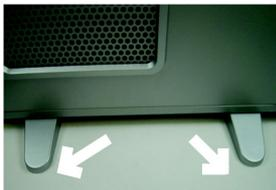
4-11-1 Swivel these four feet by 90° as shown in the figure to loosen the feet.
