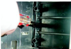
4-6-1 Open the front panel, remove the 5.25" plastic drive rail and internal metal panel.
