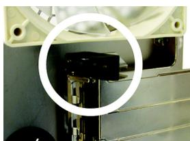
4-3-1 Open the PCI slot retention lock.
