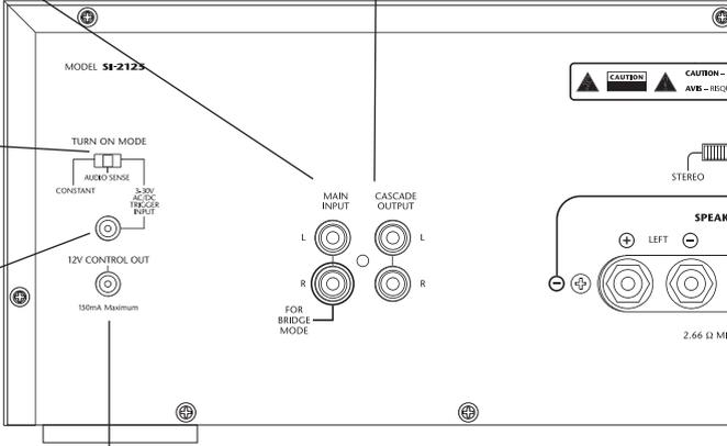
3.5mm Mini Plug socket for 12v DC Control output.
