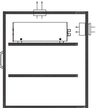
If the cabinet rear is not open to fresh air or if you're using low impedance loads, install two "boxer fans" to provide continuous air flow into and out of the cabinet.
