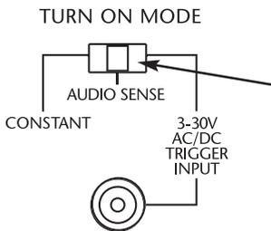
Slide the switch with your fingernail or a 1/8" slotted screwdriver blade.
