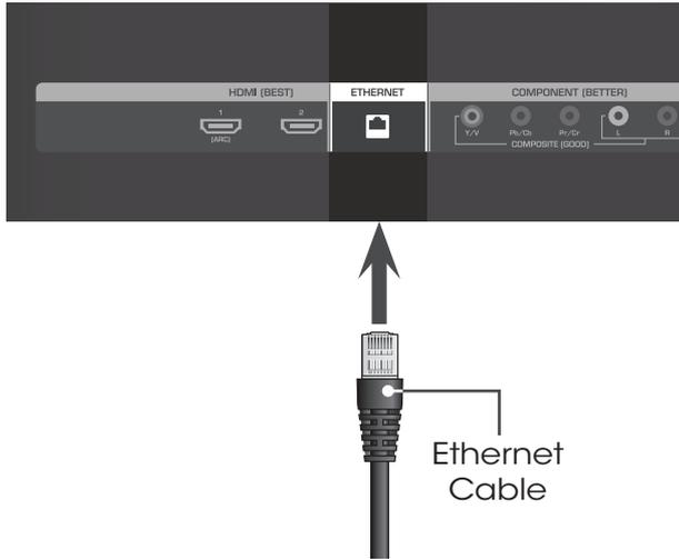
If you have a high-speed internet connection, connect an Ethernet cable from your modem or router to the back of the TV as shown.
