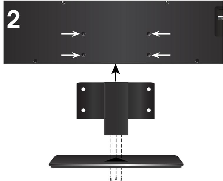
Align the base with the neck piece and tighten three (3) of the included Phillips screws with a Phillips screwdriver as shown.
