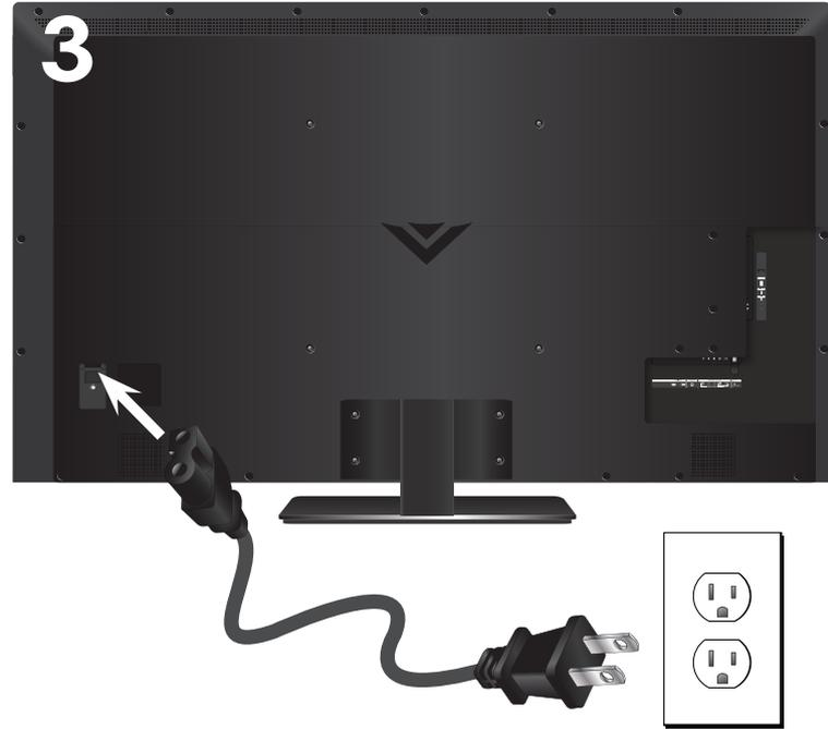
Connect the power cord to the back of the TV. The flat edge of the connector goes toward the outside of the TV.
