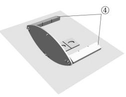
Insert two metal pegs (G) into Top Panel (A)
