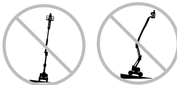
Do not raise or extend the boom unless the machine is on a firm, level surface.
