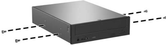
**NOTE:** There are a total of eight extra guide screws on the front of the chassis. Four have 6-32 standard threads and four have M3 metric threads. Standard screws are used for hard drives and have a silver finish. Metric screws are used for all other drives and have a black finish. Make sure to install the appropriate guide screws into the drive.
