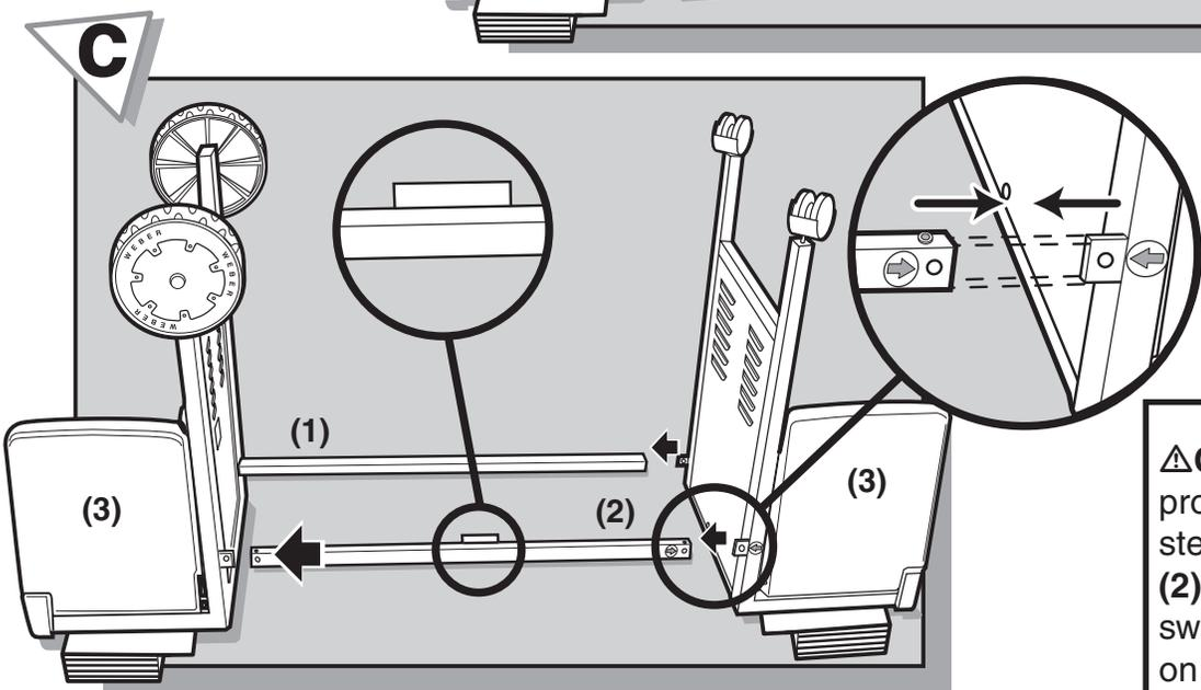
**⚠ CAUTION:** Before proceeding to the next step check that frame rail (2) is on the side with the swing tables (3). The tab on frame rail (2) must be facing toward the wheels.
