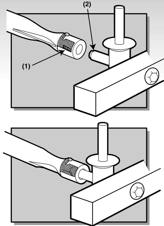
Check proper assembly before fastening manifold in place.
