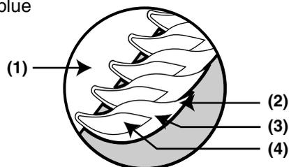
If the flames do not appear to be uniform throughout the burner tube, follow the burner cleaning procedures.
