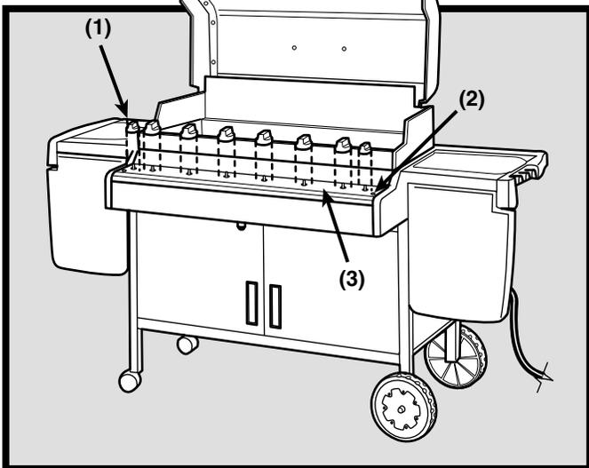
Put your fingers under the front edge of the control panel and lift off.
