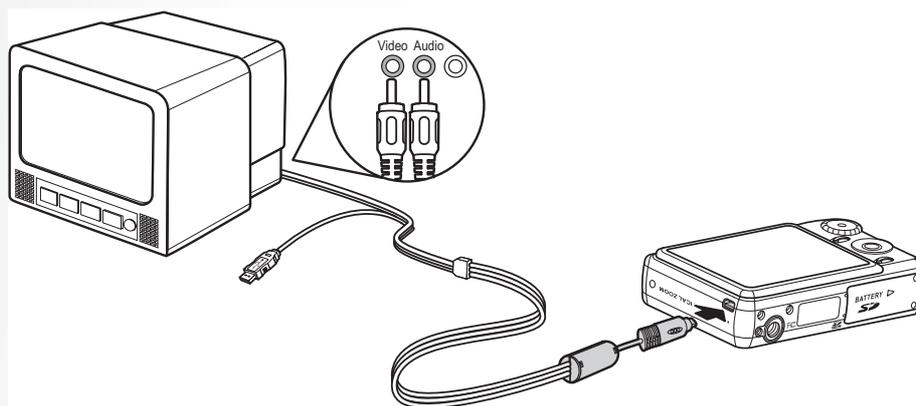
4. The LCD screen turns blank and all images and video clips are displayed on the TV screen. Follow the same steps described in "Viewing Photos/Videos on the LCD Screen" on page 27.
