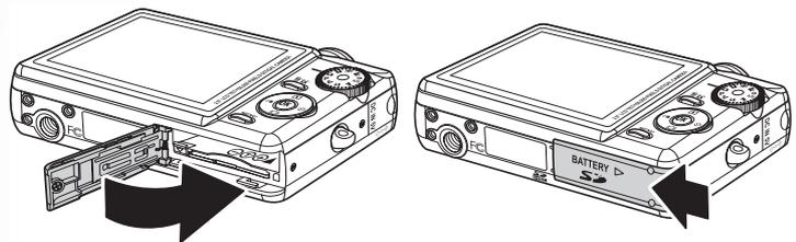
To remove the SD/MMC card, gently push the card until it pops out. Pull out the card carefully.
