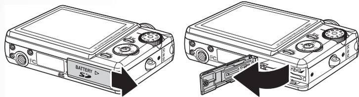
2. Insert the SD/MMC card into the memory card slot as shown.
