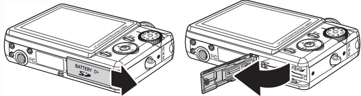
2. Insert the battery into the compartment observing the correct polarity.
