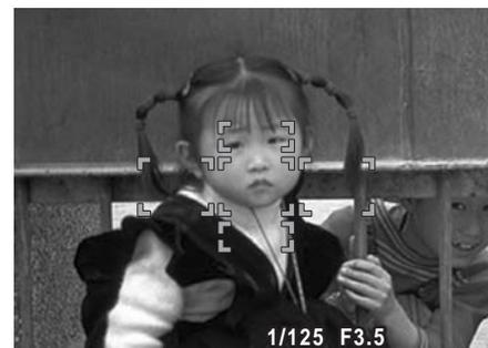
However, when the camera fails to detect your subject's face, the camera will set the focus to **Multi-Zone** with a green or red focus frame.
