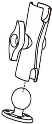
4. Tighten the arm turnscrew until the U-bracket is secured to the RAM arm and the vehicle.
